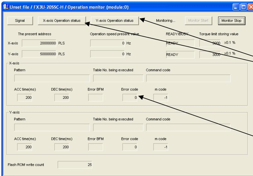
These buttons provide detailed information on the operation speeds and addresses. They also allow monitoring of servo speeds in RPM.
