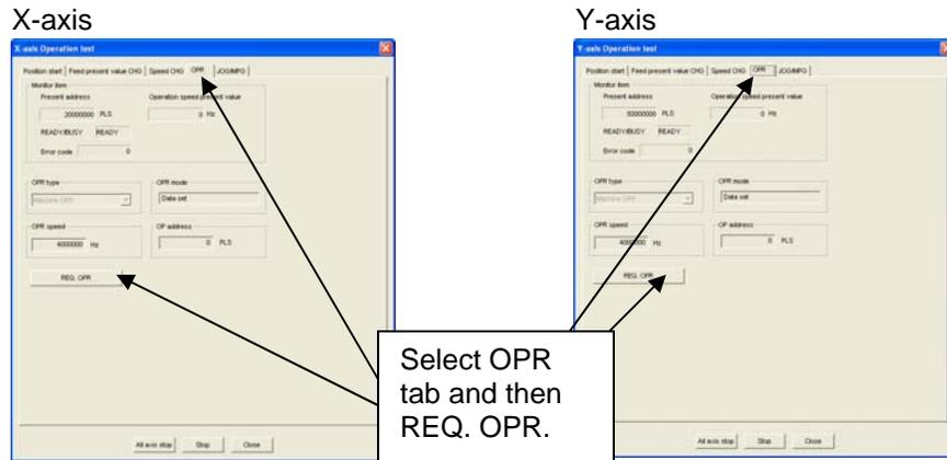
Since the mechanical zero return mode has been set to the data-set type from *Section 4.1: Initialization Process*, the value in BFM# 14028, 14029 (initially zero) is directly written to the current address.
