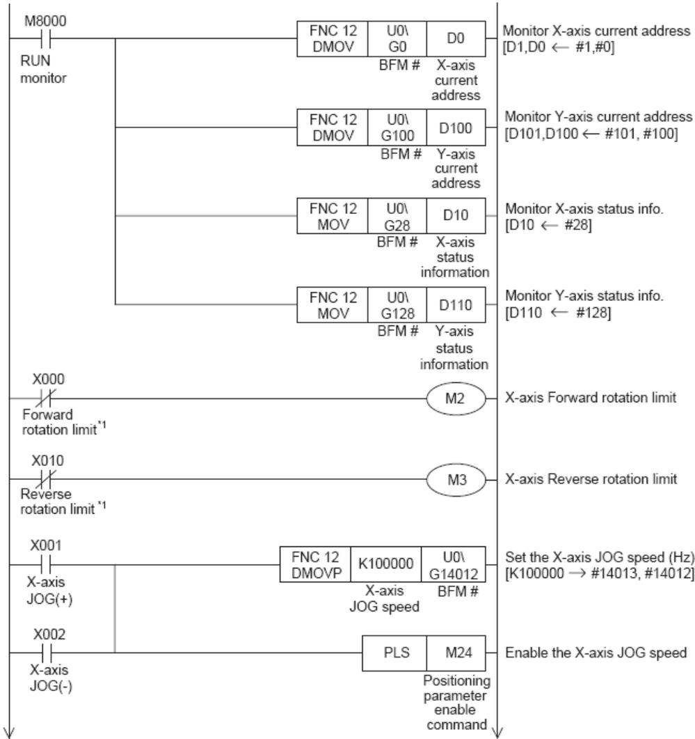
\*1. The forward and reverse rotation limit switches must be wired so that they are turned ON by default. When these limit switches turn OFF (due to the workpiece going out-of-bounds), M2 or M3 will turn ON and cause the pulse operation to stop.
